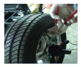
13) Rotate the wheel until all the indicating lights on the "inner" side of the display are fully illuminated and then add the 100g calibration wheel weight to the inside of wheel at the 12 o'clock position
