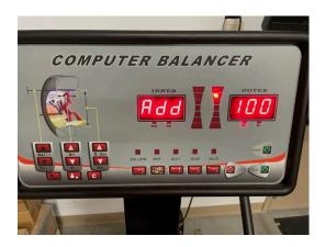
10) Manually rotate the wheel until all indicating lights on the "outer" side of the display are fully illuminated and then add the 100g calibration wheel weight to outside of wheel at the 12 o'clock position
