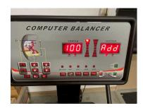
12) Remove the 100g weight from the outside of the wheel
